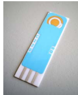
C220AT High temperature curing ink, WE 4mm. Work in solution (sensing area closer to the end of the strip)
