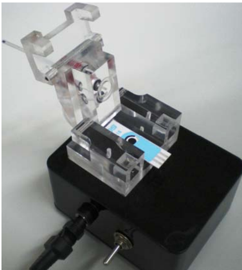
A switch allows to easily turn on and off magnet
