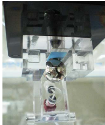
Image shows the strong attraction applied to the SPE's sensing area by the potent magnet.
