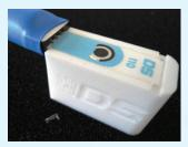
Also, specific **connectors** that act as an interface between the screen-printed electrode and any potentiostat (refs. DSC, CAC) are available at *DropSens*.
