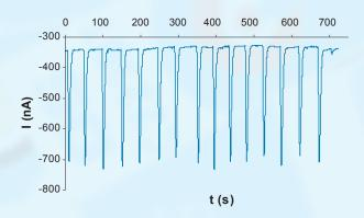
Amperometric detection of hydrogen peroxide in a flow injection analysis system with our easy to use Flow-cell. The amperometric responses for  $1\cdot 10^{-4}$  M  $H_2O_2$  at a ref. 710 electrode do not show any fouling effect. RSD% = 3.2, n = 15.
