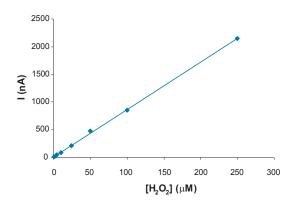
Calibration curve for hydrogen peroxide (in a 0.1 M phosphate buffer pH 7.2) from  $1\cdot10^{-6}$  M to  $2.5\cdot10^{-4}$  M in a FIA system (ref. FIASYSTEM using our Screen-printed Co-Phthalocyanine/Carbon electrodes. E<sub>det</sub> +0.4 V; Flow rate 2.2 ml/min
