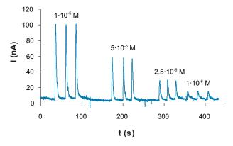
Amperometric detection of hydrogen peroxide in a flow injection analysis system with our easy to use flow cell (ref. FLWCL). The amperometric responses for decreasing  $\rm H_2O_2$  concentrations at a ref. 410 electrode show neither fouling nor memory effects.  $\rm E_{det}$  +0.4 V; Flow rate 2.2 ml/min; Flow carrier 0.1 M phosphate buffer, pH 7.2
