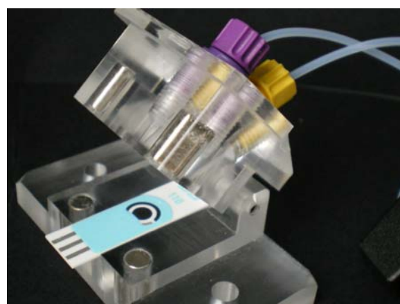
Figure 4. Flow-cell for screen printed electrodes
