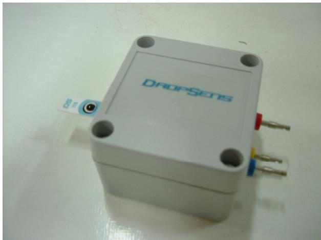
Also a specific **connector** (ref. DSC) that acts as an interface between the screen-printed electrode and your potentiostat is available at [DropSens](#).
